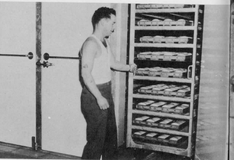
After rising in the steam room, the bread is ready for the oven.
